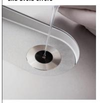
Micro-volume UV/VIS measurement is the method of choice when measuring either small sample amounts or high absorption samples. Only 1 µL of sample is required for reliable measurements. The pure sample is pipetted on the measuring surface and the arm is locked automatically to a precisely defined pathlength. Measurement errors are avoided, as the sample does not need to be diluted.
