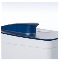
LockPath enables the measurement of wide concentration ranges from 6 to 15,000 ng/µL of dsDNA without further dilutions within 2 seconds per pathlength. The most suitable pathlength can be automatically locked. The arm design prevents the sample from drying out during measurement, significantly increasing repeatability.
