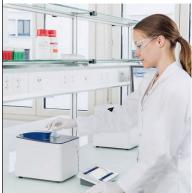
The UV5Nano combines two instruments in one for microvolume and cuvette based measurements. Once the arm is at a 90 degree position, the measurement surface can be easily accessed with a pipette from either the left or the right. The curved lid on top of the instrument allows convenient positioning of the operator's hand to securely guide the pipette tip.
